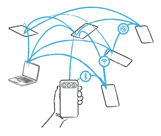
qaul provides a solution for a **secure local off-the-grid peer-to-peer communication**. Devices can interconnect and communicate via **Bluetooth**, **Wifi**, **LAN and via Internet** overlay. All interconnected devices are meshed together.
